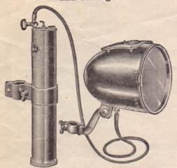
For Motor Cycles, Yachts and Boats. Will fit any Motor cycle. The generator holds 8 oz. carbide, 11 inches long and 2 inches in diameter. Made of heavy brass, nickel-plated. Carbide chamber equipped with grating for separating used from unused carbide. Will work in an upright position or at an angle
