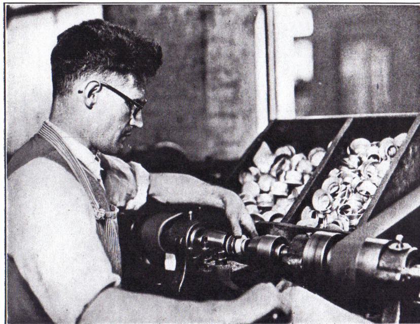
Putting a corrugated knurl around the edge of the carbide container.
