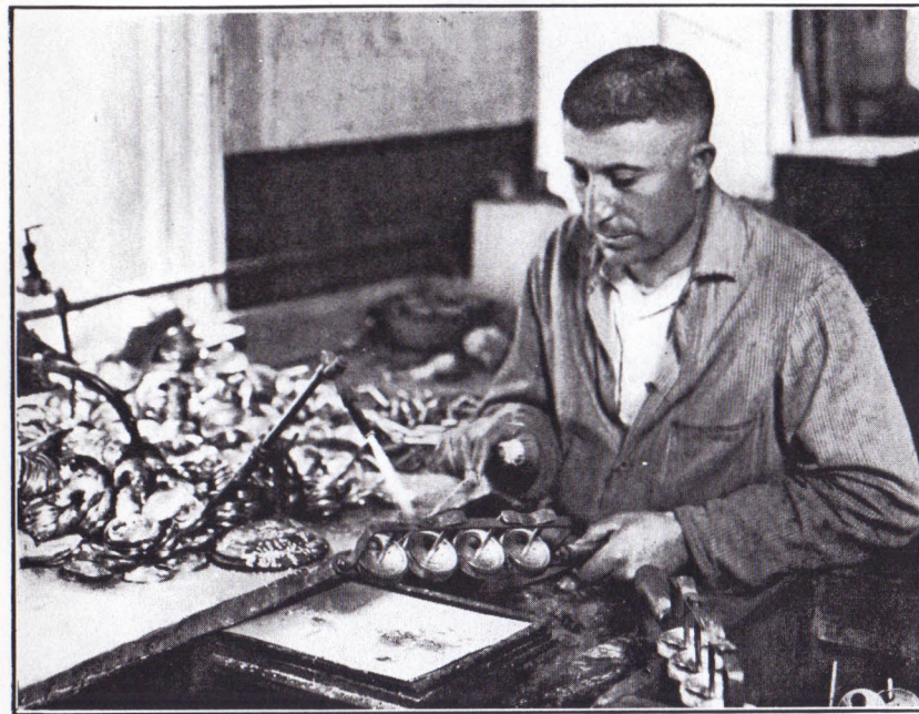
Soldering the water tube by gas torch to the inside of the top cover.
