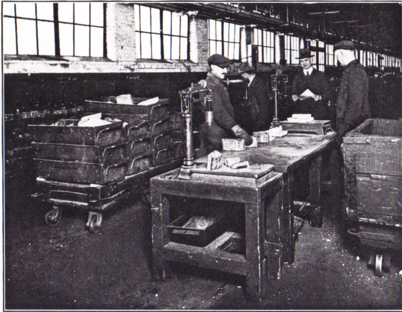
Weighing out the correct amount of copper and zinc for a certain brass alloy.
