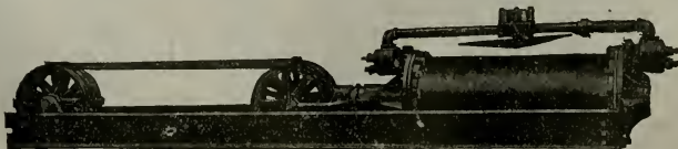
Fig. A. D. 603. Stationary Class "K" Hoist with Cushions and Speed Boxes
